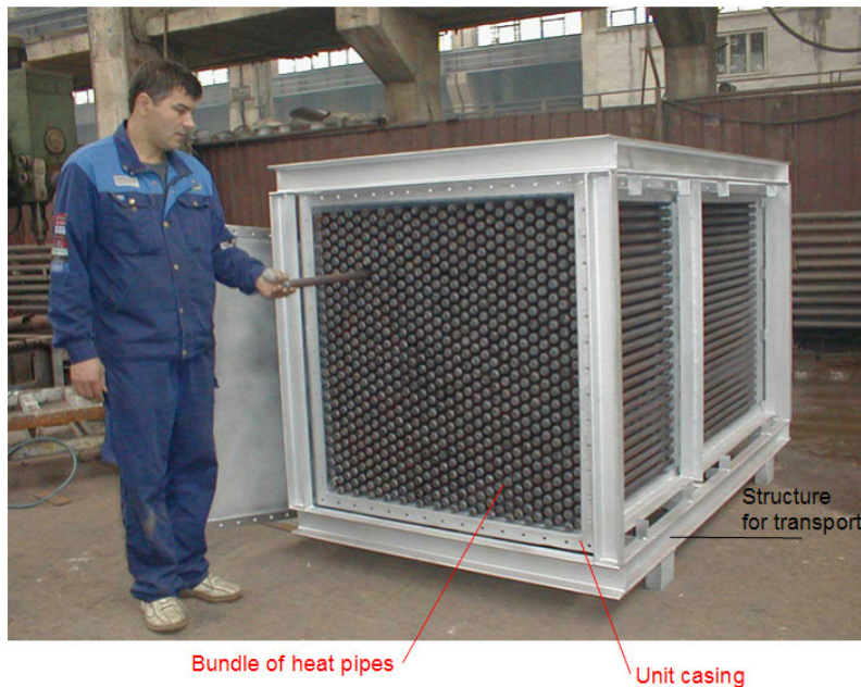
Figure 1 - Econotherm® GA units can be easily cleaned by simple pipe removal
