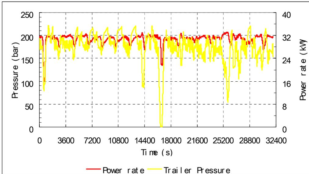
Figure 7 - Power rate and the trailer pressure
