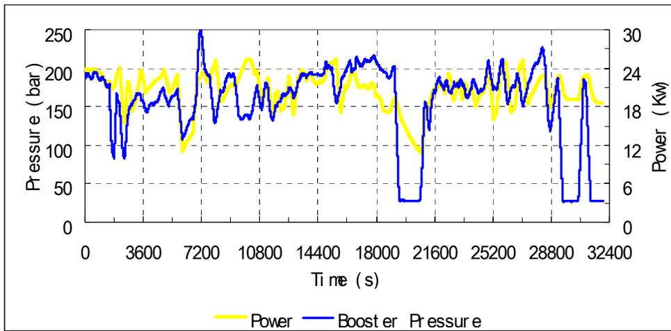
Figure 2 - Power and Booster Outlet Pressure for Booster #1
