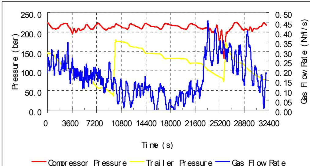
Figure 5 - Compressor station pressures and flow rate
